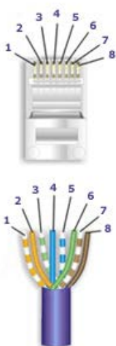
568-B Wiring Diagram The most common wiring scheme
